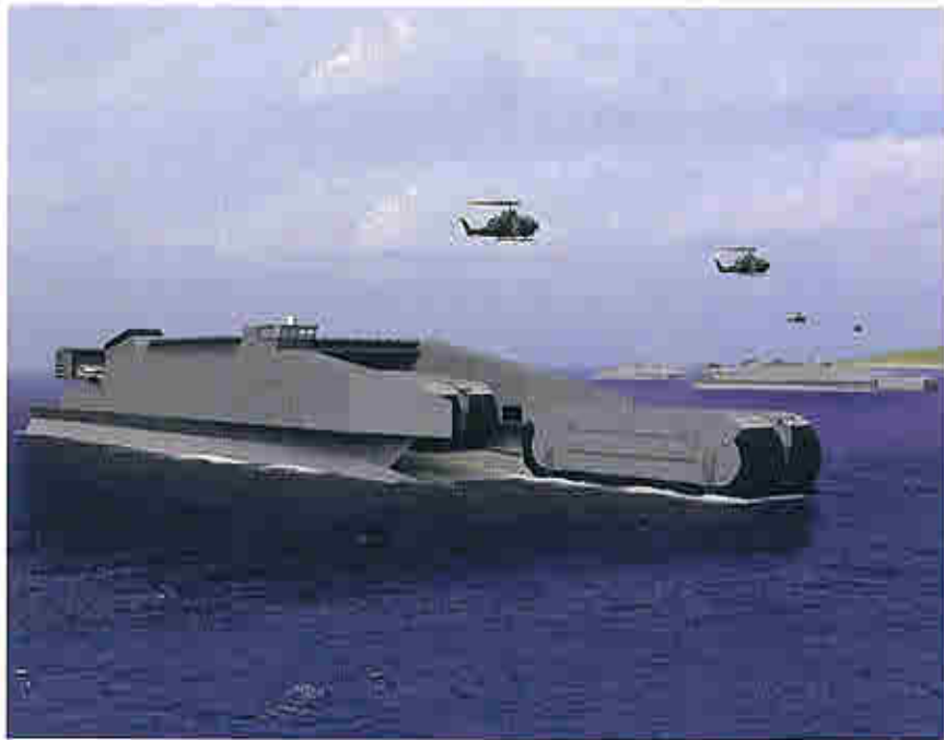
Artist's concept of the T-Craft with the Captive Air Amphibious Transport (CAAT at the bow).
